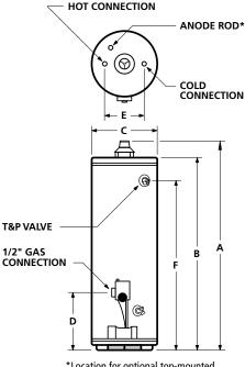
\*Location for optional top-mounted T&P Valve if ordered from factory.
